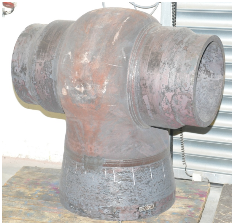
Valve built of forged plate, large sizes possible.
