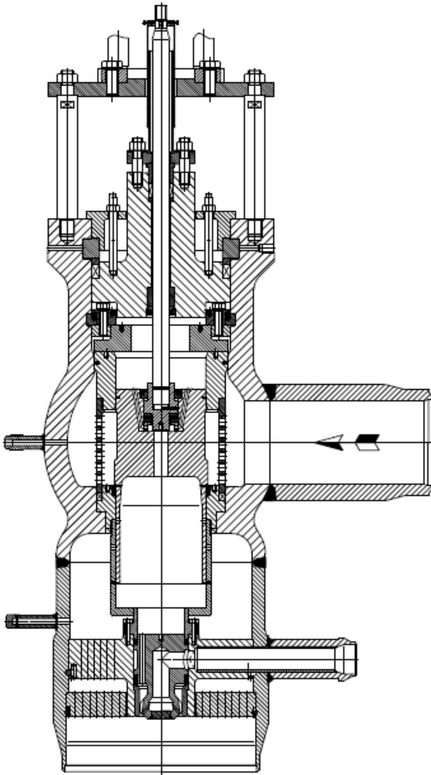
*Ball shaped PRDS made of forged material equipped with a pressure seal, perforated cages with a pressure balancing system and an integrated steam atomizing unit*
