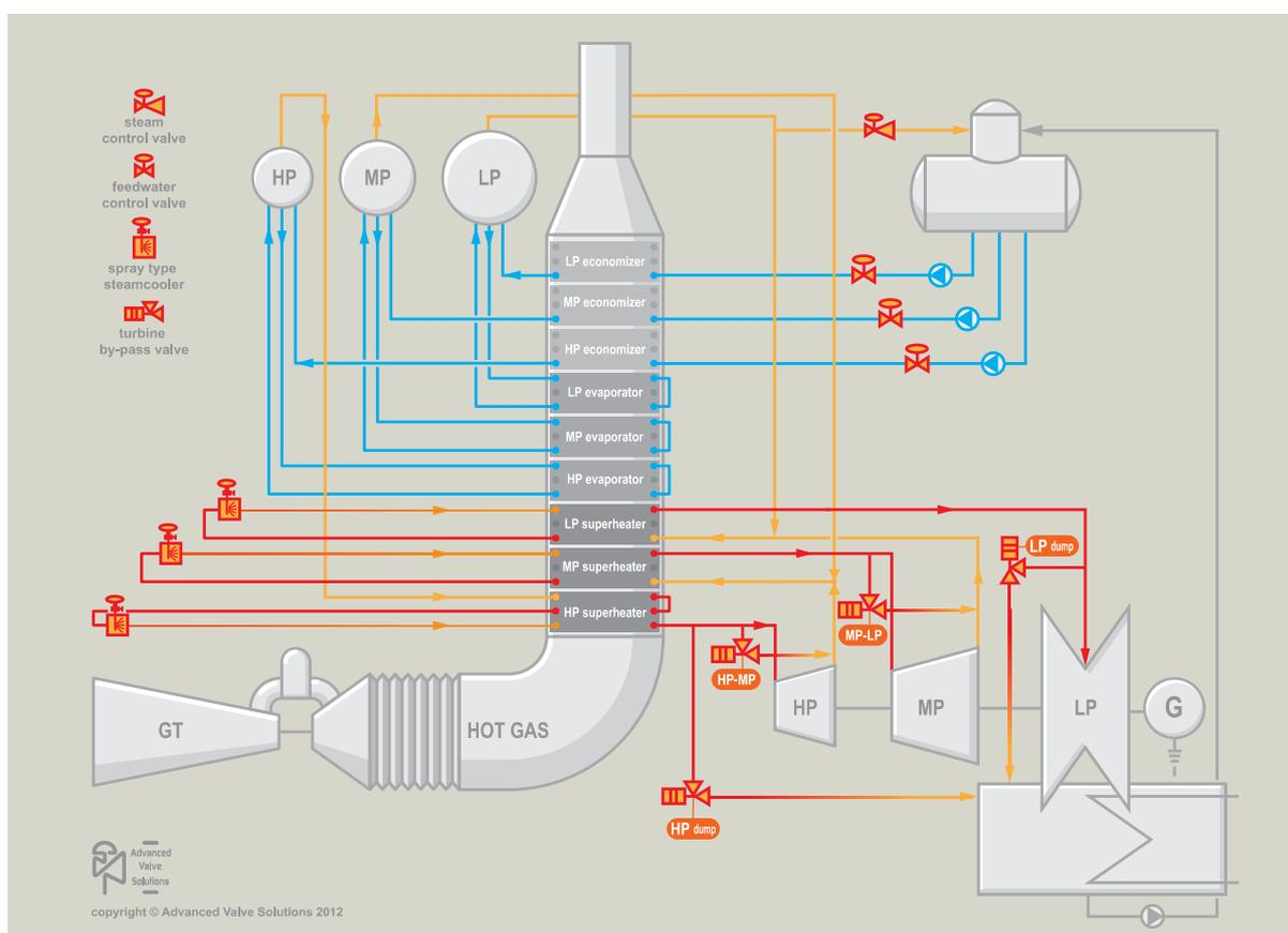
basically a control valve with an integrated spray water steam cooling facility.
