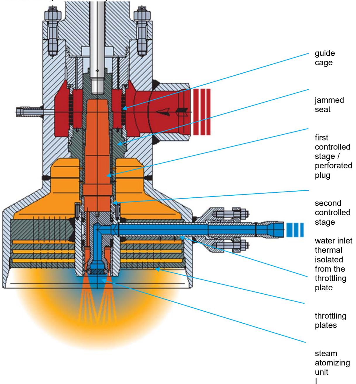
In the show valve above we see a 6 stage pressure reduction, based on 2 controlled stages and 4 throttling plates. The steam cooling is done with a steam atomizing unit, positioned in the centre of the valve. The valve body is based on a forging, bolted bonnet, and a jammed trim for easy maintenance.
