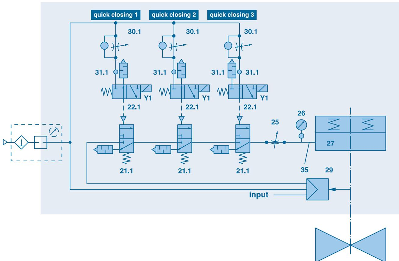
*Schematic showing a quick closing device based on EN 12952-3 / TRD 421. The 3 quick pneumatic valves discharge the air from the “spring to close” pneumatic actuator and are also closing the air supply from the positioner when the quick closing valves are activated.*
