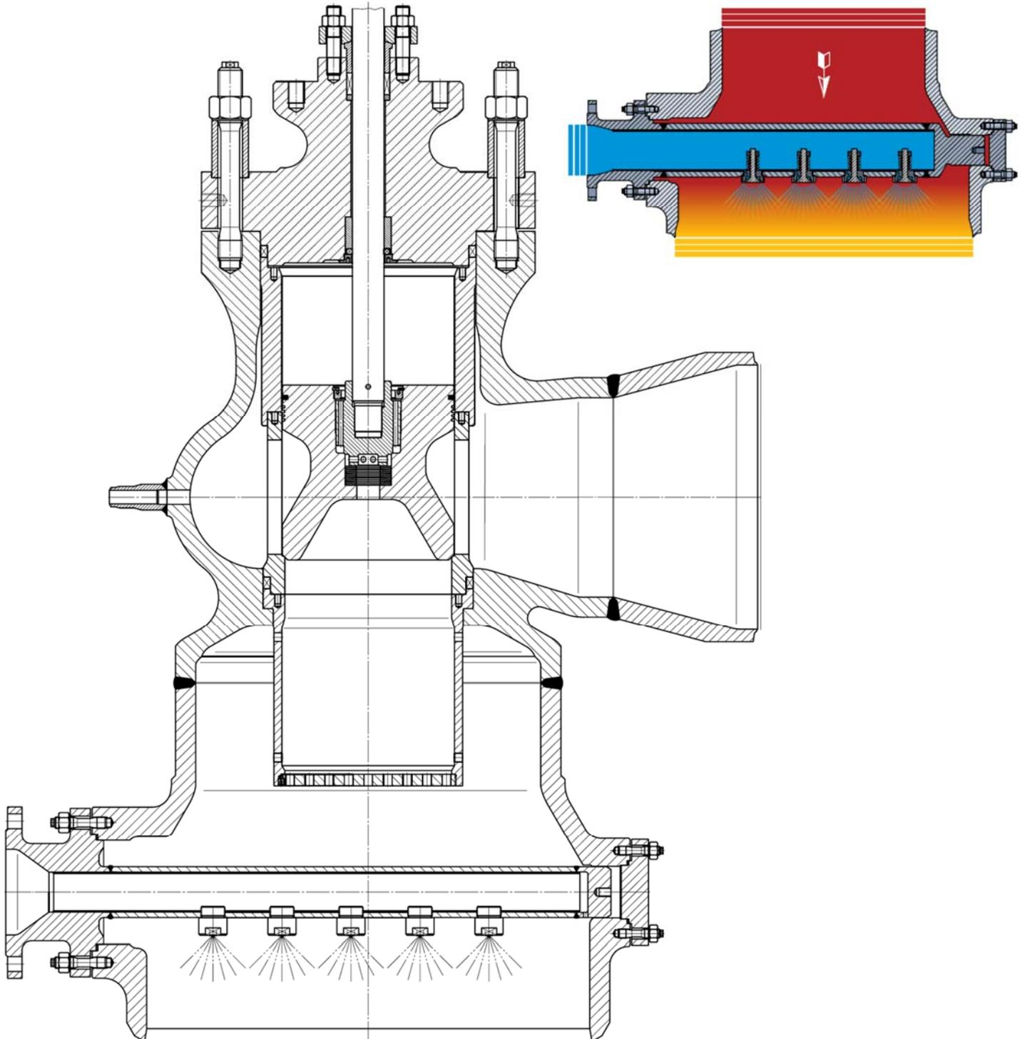
*LD turbine bypass, cast body, balanced plug, outlet cone with spring loaded nozzle type water injection.*
