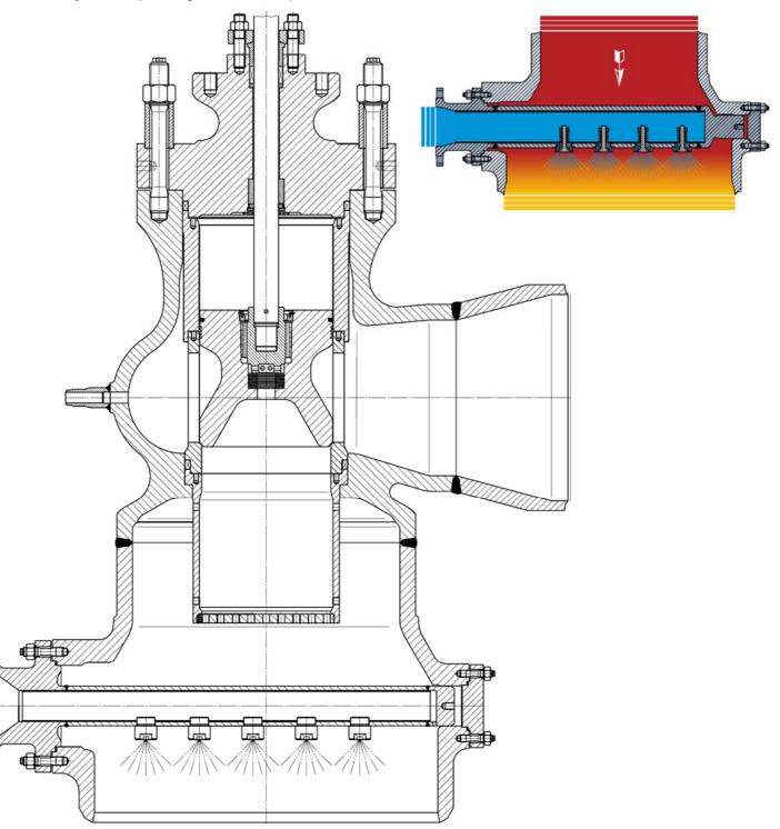
LD turbine bypass, cast body, balanced plug, outlet cone with spring loaded nozzle type water injection.
