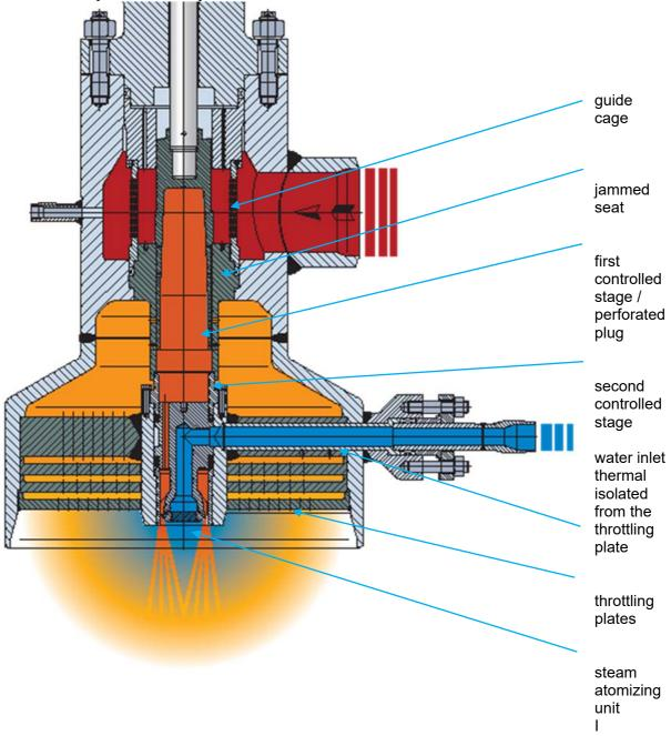
In the show valve above we see a 6 stage pressure reduction, based on 2 controlled stages and 4 throttling plates. The steam cooling is done with a steam atomizing unit, positioned in the centre of the valve.
