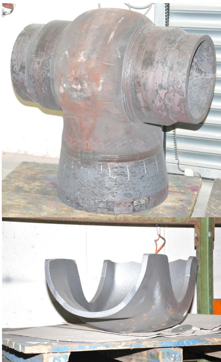
Valve built of forged plate, large sizes possible.
