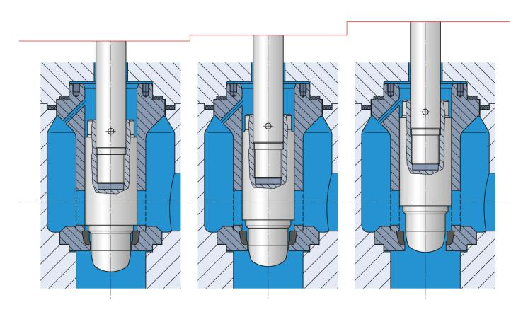
Clamped trim, separated seat and control area.
