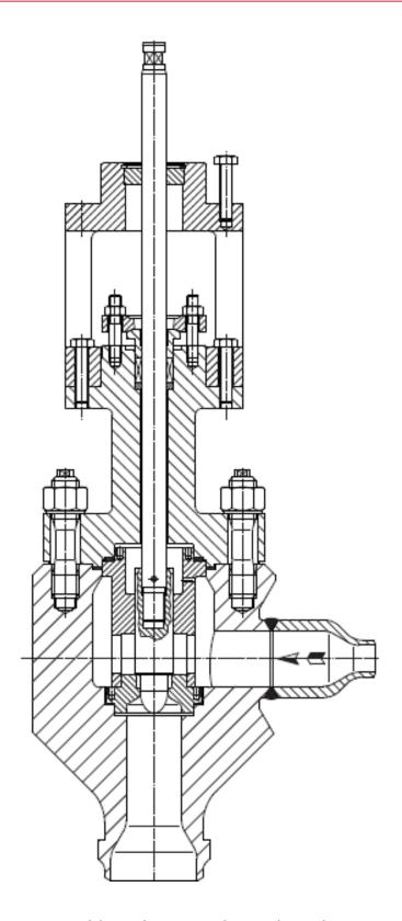
Typical drain valve, separated seat and control, clamped trim, forged body, increased diameter at the outlet.
