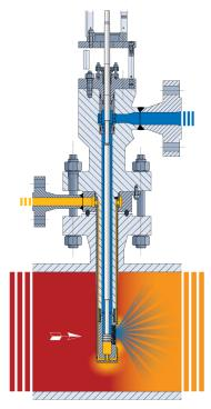
shock. A saturated steam flow is bypassed from the superheater and is fed into a cooling jacket keeping the attemporator body at a low temperature level. The cooling steam is mixed up again with the main steam, resulting in no influence on the installation efficiency.
