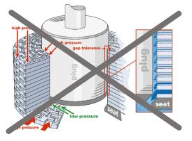
Due to uncontrolled gap flows staggered trims are failing.
