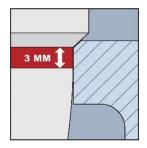
The first part of the stroke does not control any flow but is just energizing the different control stages. Moreover is it avoiding hammering during opening.
