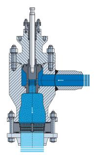
Throttling plates can be used to control the flow between the valve and the drain vessel.
