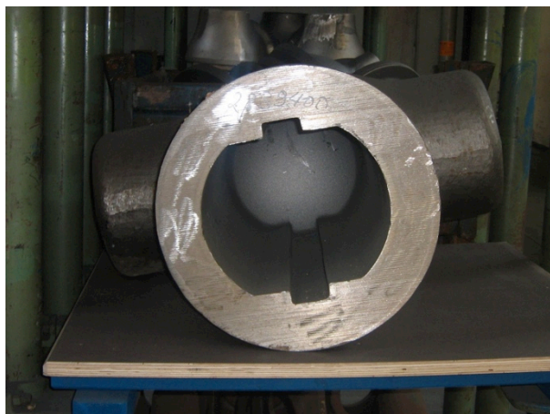
ABOVE LEFT AND RIGHT: Hollow forged valve bodies.
