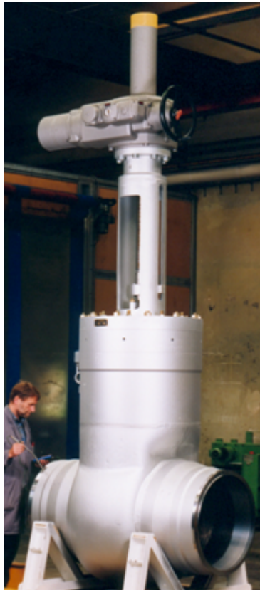
One of the installed valves in the UK in a HRSG reheat application has performed 100.000 cycles without any problems.
